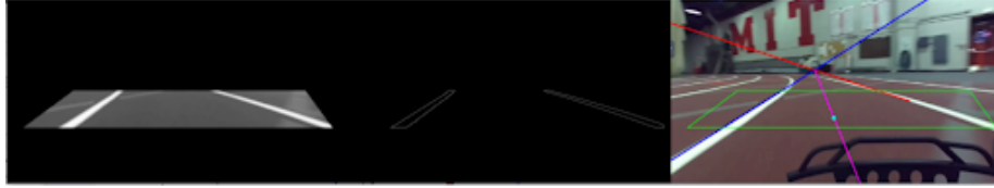
Figure 2: Sequence of images showing pursuit point image processing. The leftmost image shows steps 1 and 2. The center image shows step 4. The rightmost image shows steps 4-8, where the blue line is the left lane line, the red line is the right lane line, the pink line is the pursuit line, and the aqua dot is the pursuit point.
